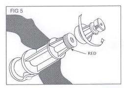
2. Connect the hot outlet thread (RED) to the breathing tube and tighten by hand (Fig 6). Connect the regulator to the cold outlet.
