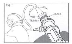
2. Connect the air supply hose to a breathing air source, supplying EN 12021 or better quality air. Connect the air supply hose to the Blastrite CCT quick disconnect plug.
